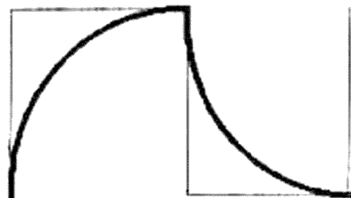
Square Wave before and after Lag Processor
