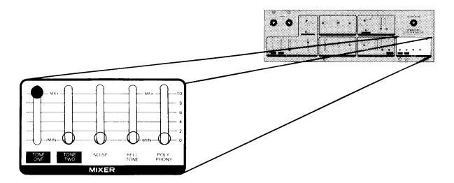
The **MIXER** is to the right of the **FILTER** section. It blends all the different possible sources of sound. So far, you've only used a single source (**TONE ONE**) to create the sounds. We are going to broaden a few horizons right now.
