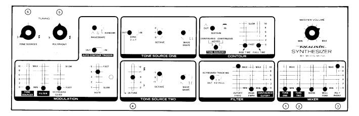
Adjust the controls on your synthesizer to exactly match the diagram. **MASTER VOLUME** should be adjusted to a comfortable sound level. Notice that there are six controls specially marked on the diagram. Controls 4, 5, and 6 are **extremely** sensitive and will only require slight adjustment.
